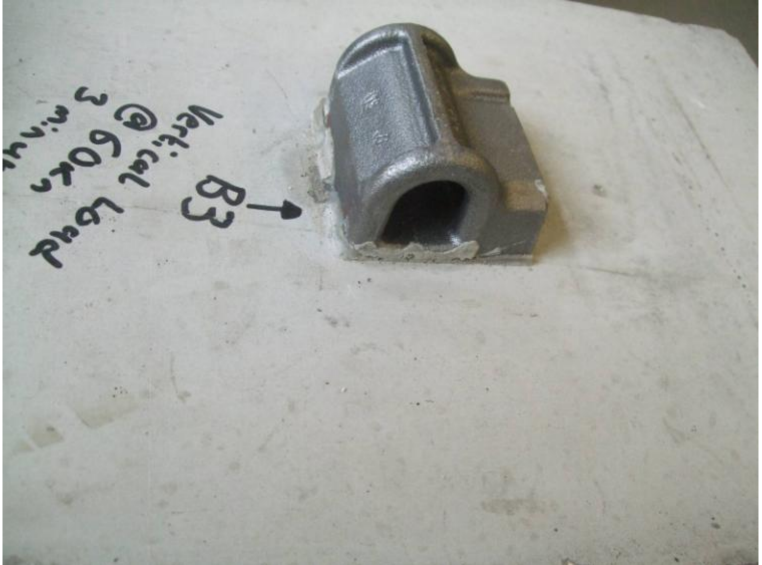
Vertical Load Test - Cast-in Component Surface after Test
