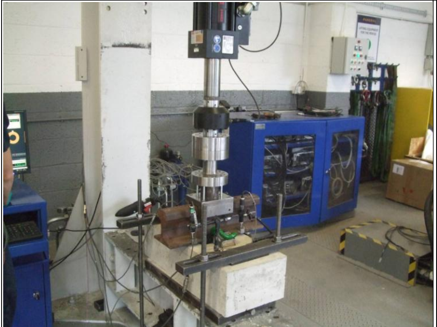
Clamping Force - 100kN Actuator Test Rig & Transducer Arrangement
