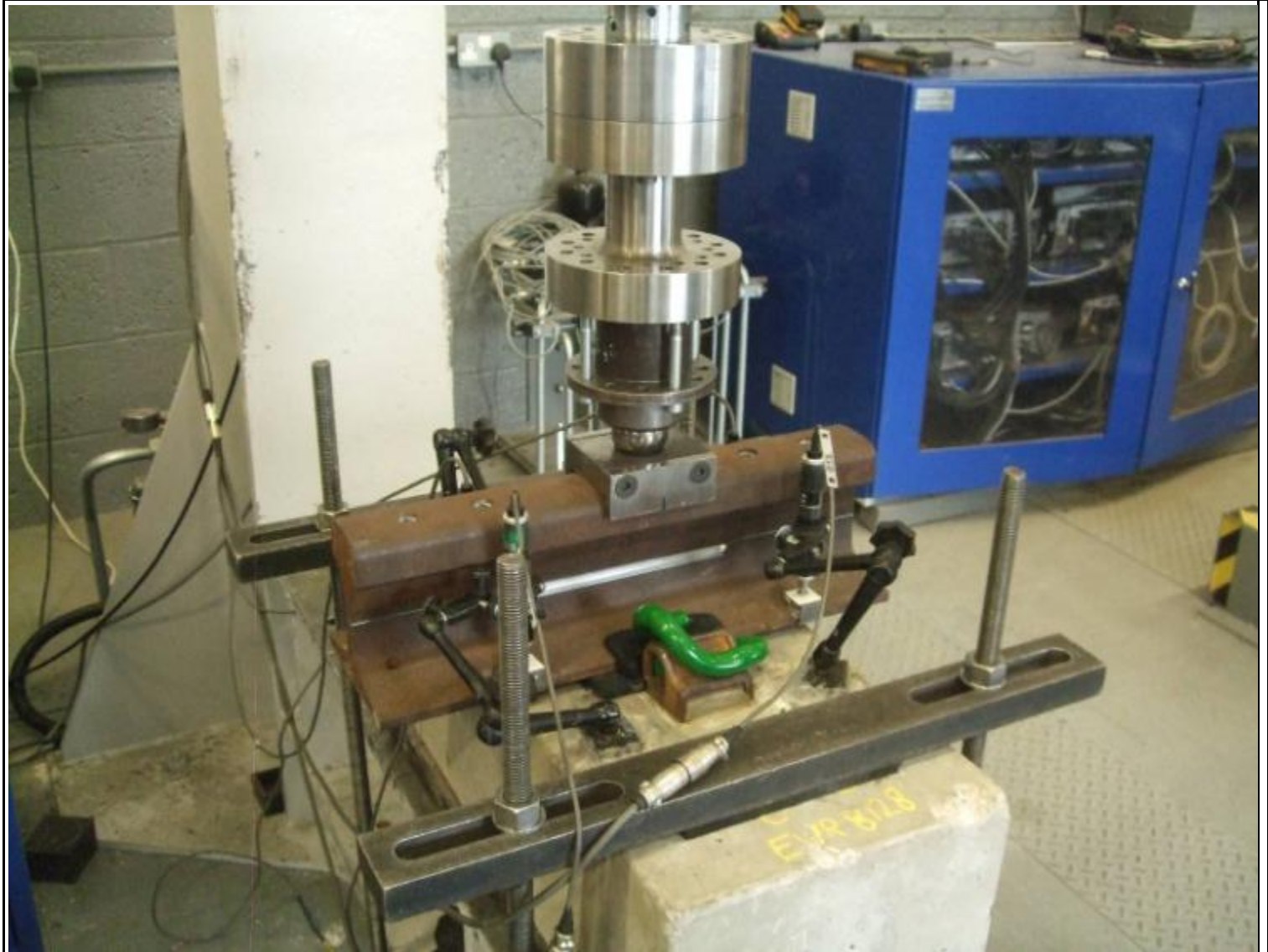
Dynamic Stiffness - 100kN Actuator Test Rig & Transducer Arrangement
