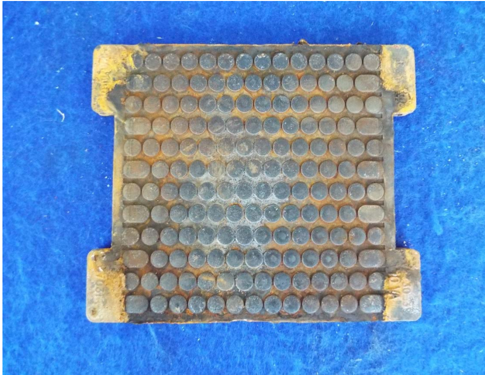
Figure A9: Rail pad upper surface following effects of severe environmental conditions test
