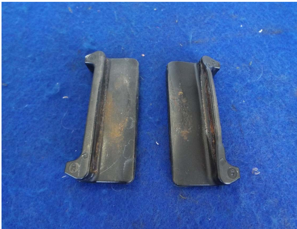
Figure A4: Insulators lower surface following repeated load test
