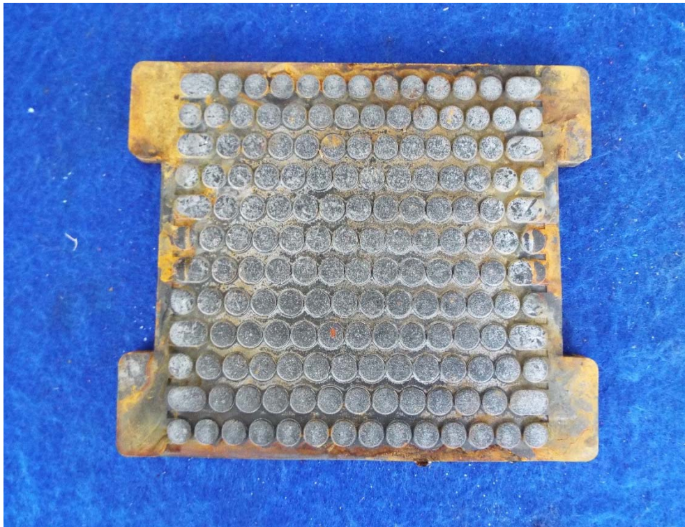
Figure A10: Rail pad lower surface following effects of severe environmental conditions test
