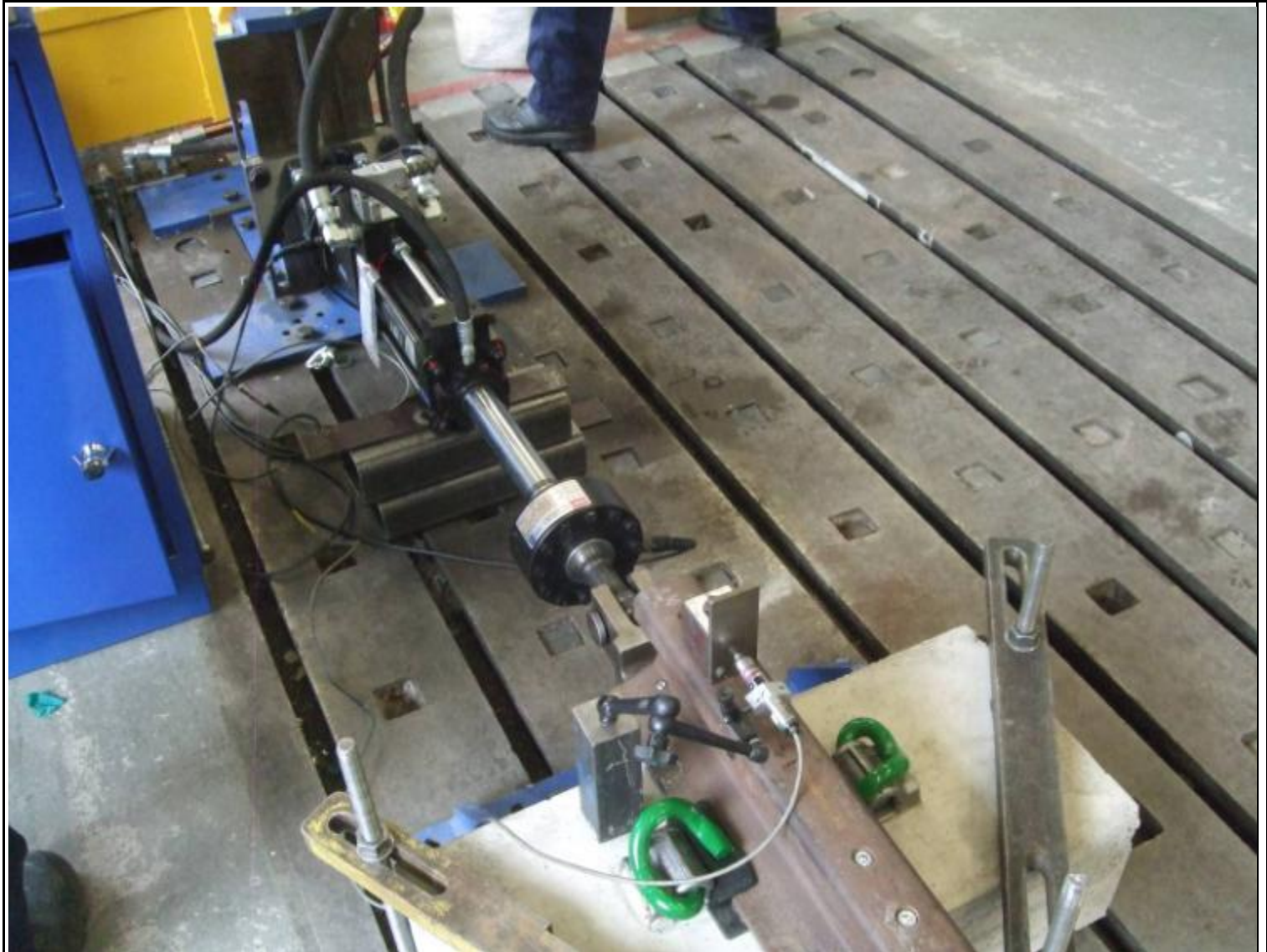
Longitudinal Rail Restraint - 100kN Actuator Test Rig
