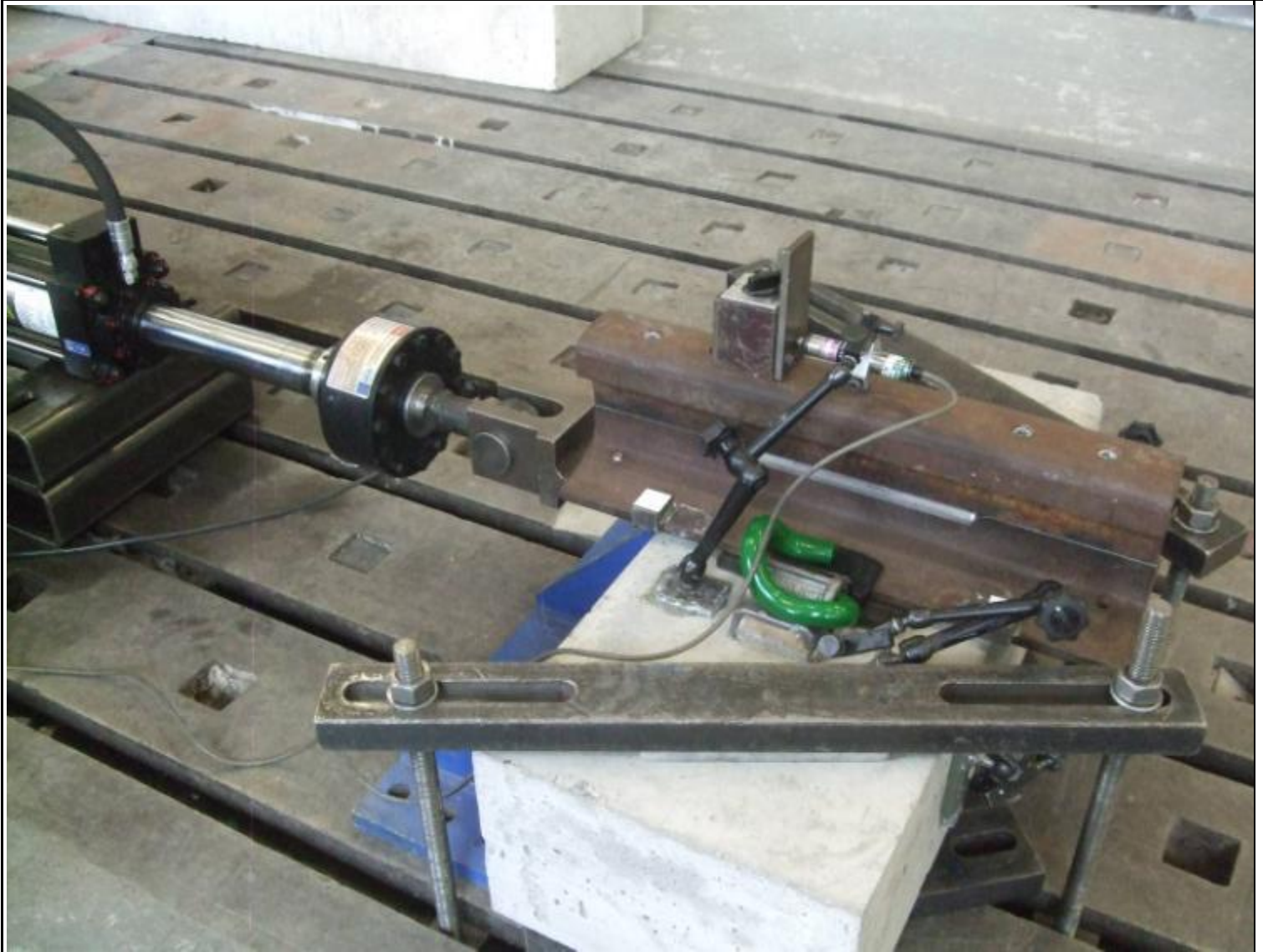
Longitudinal Rail Restraint - 100kN Actuator Test Rig & Transducer arrangement
