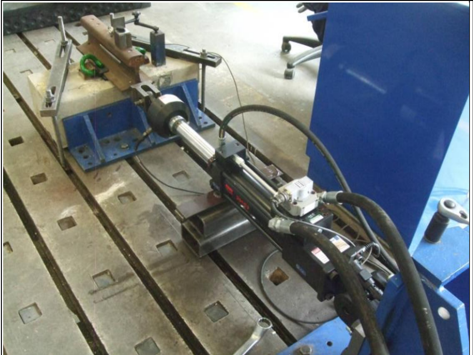
Longitudinal Rail Restraint - 100kN Actuator Test Rig
