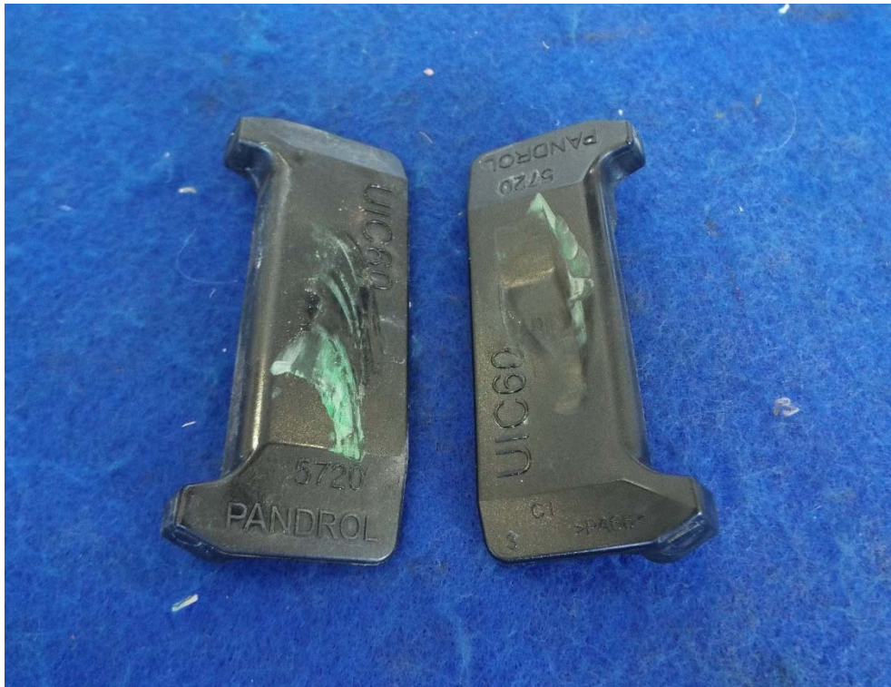
Figure A3: Insulators upper surface following repeated load test
