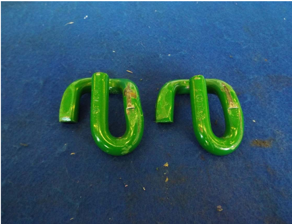
Figure A6: Rail clips lower surface following repeated load test
