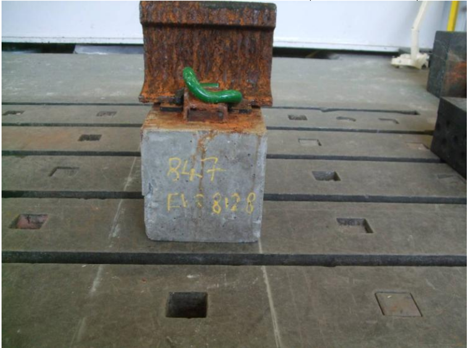
Severe Environmental Conditions - Test sample after 313 hours Immersion
