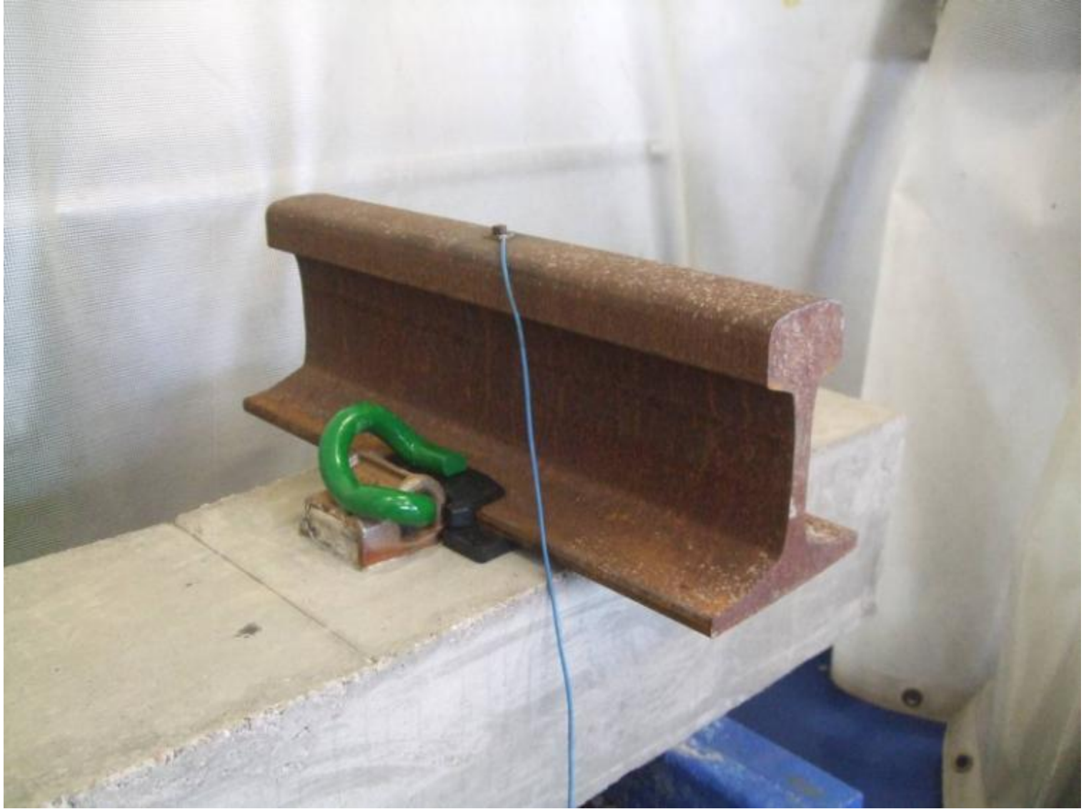
Electrical Resistance Test Sample & Electrical Connection
