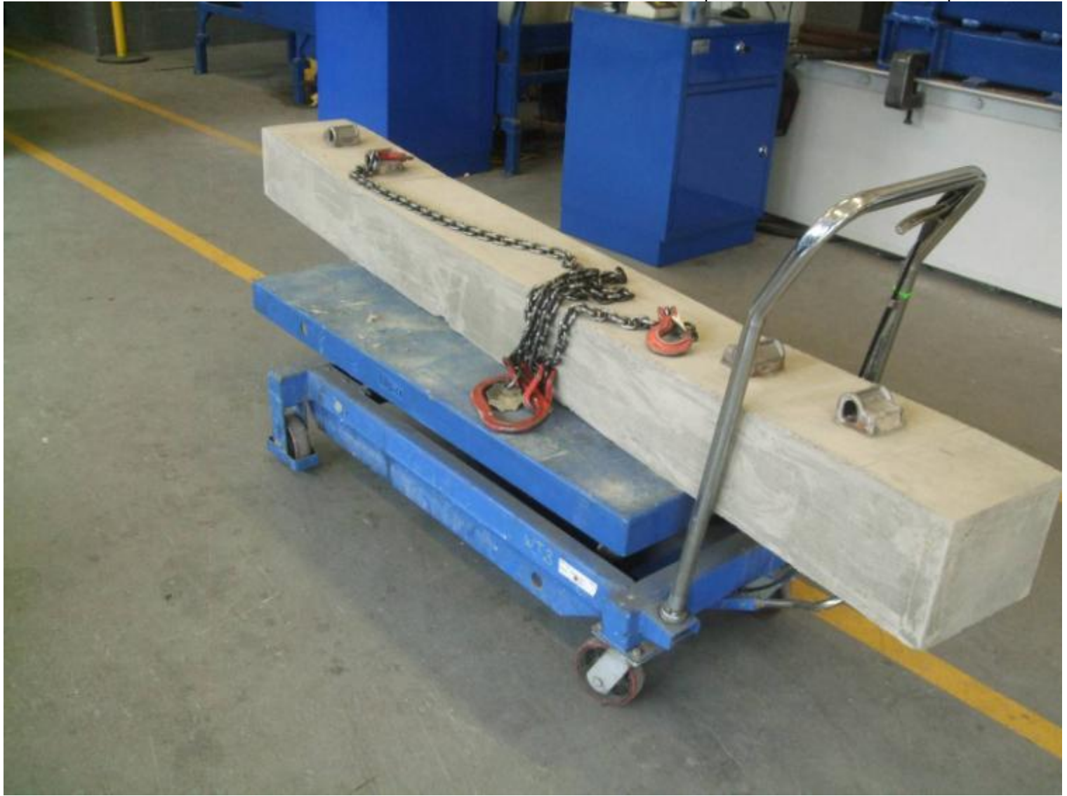
Electrical Resistance Test Slab
