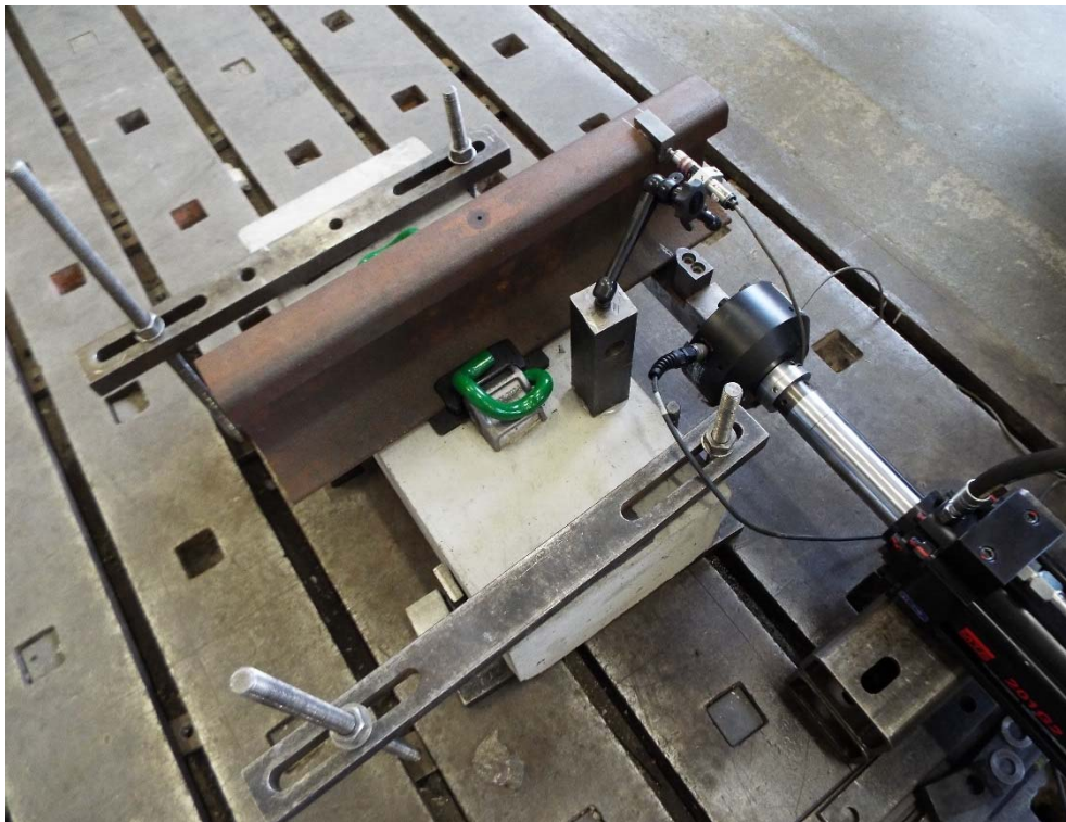
Figure 2.8.1: Torsional resistance test arrangement
