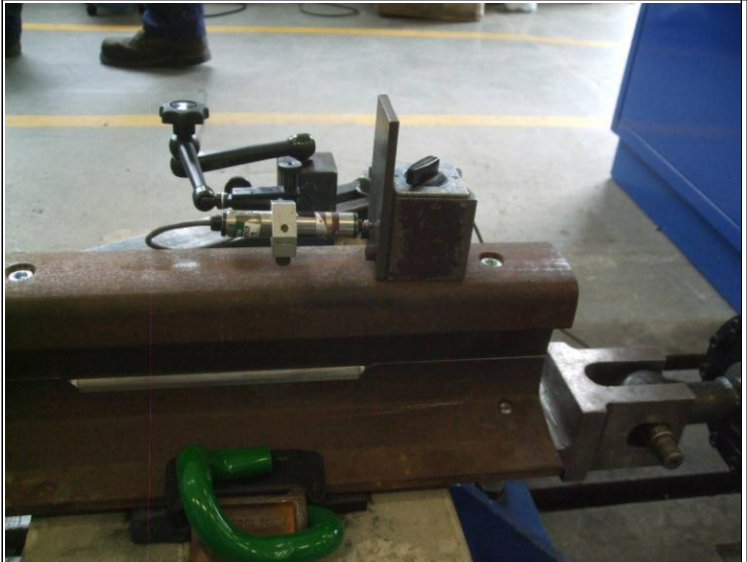
Longitudinal Rail Restraint – Transducer arrangement
