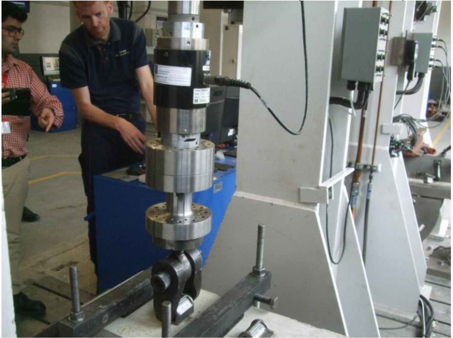
Vertical Load Test Rig – Cast-in Component
