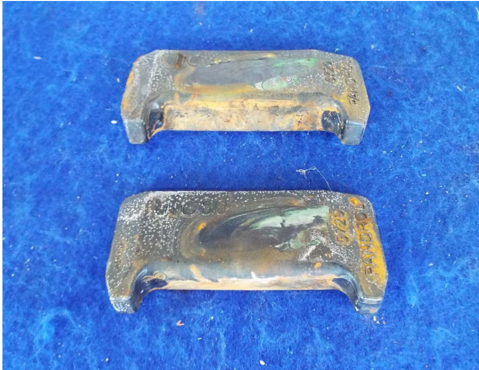
Figure A11: Insulators upper surface following effects of severe environmental conditions test
