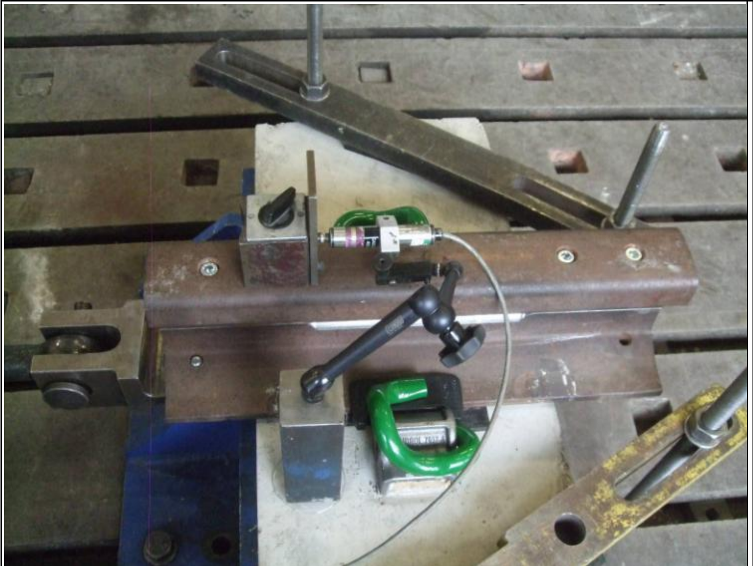
Longitudinal Rail Restraint – Transducer arrangement
