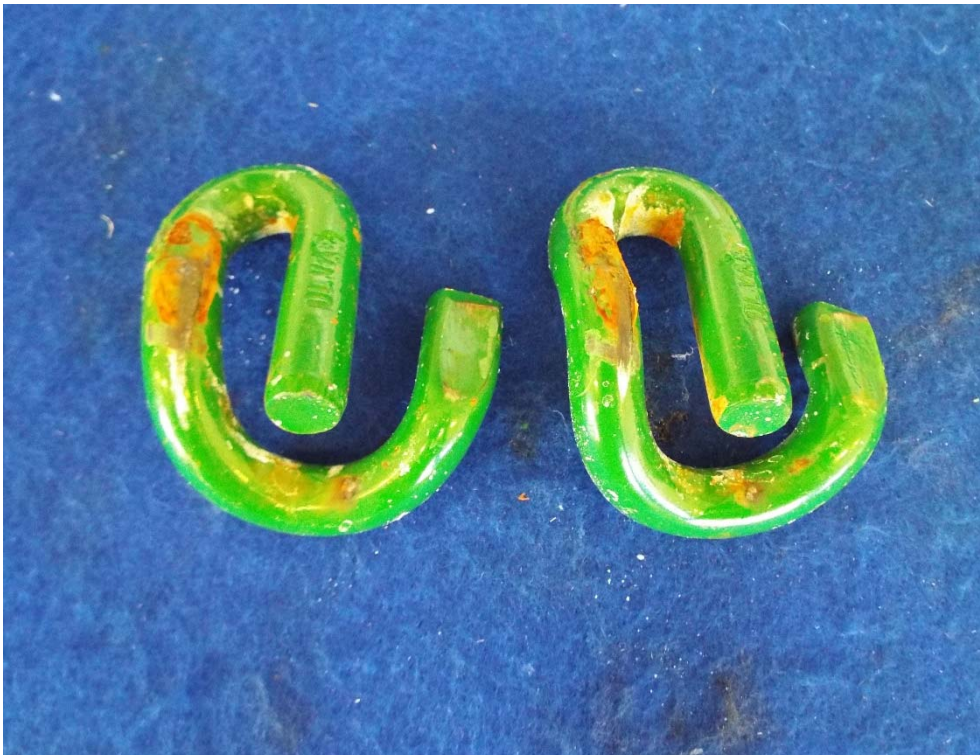
Figure A14: Rail clips lower surface following effects of severe environmental conditions test
