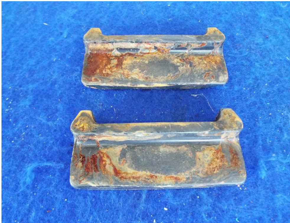
Figure A12: Insulators lower surface following effects of severe environmental conditions test
