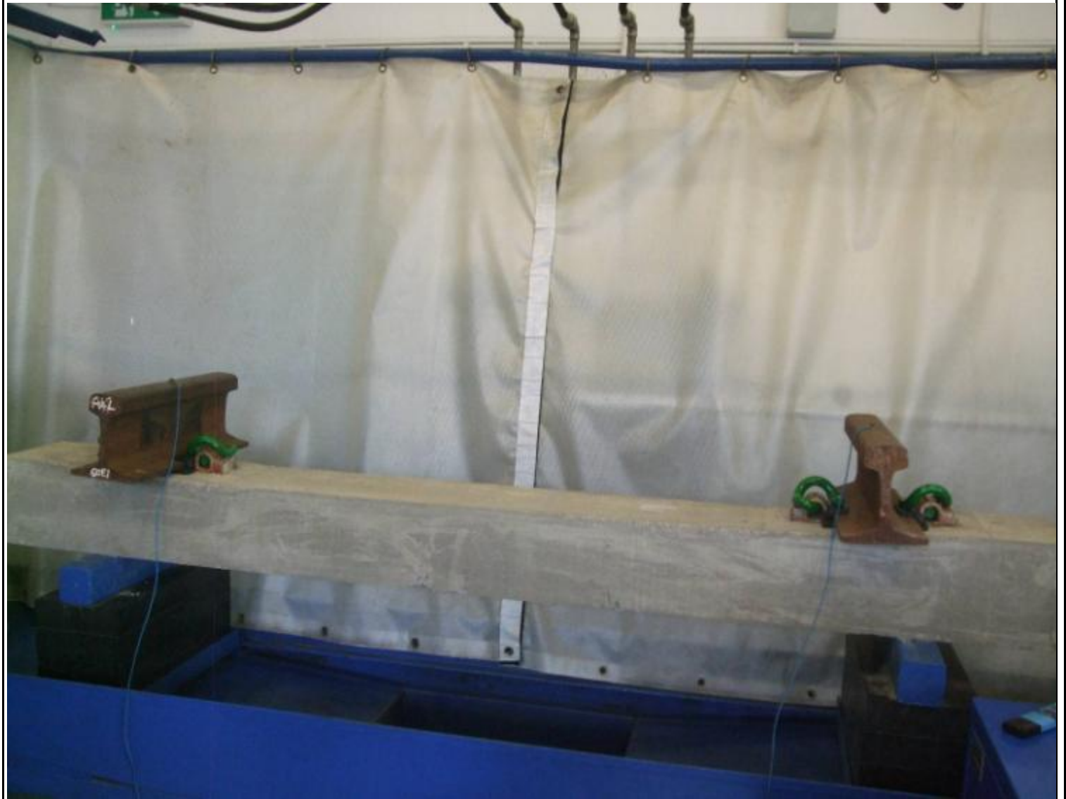
Electrical Resistance Test - Test Spray Booth
