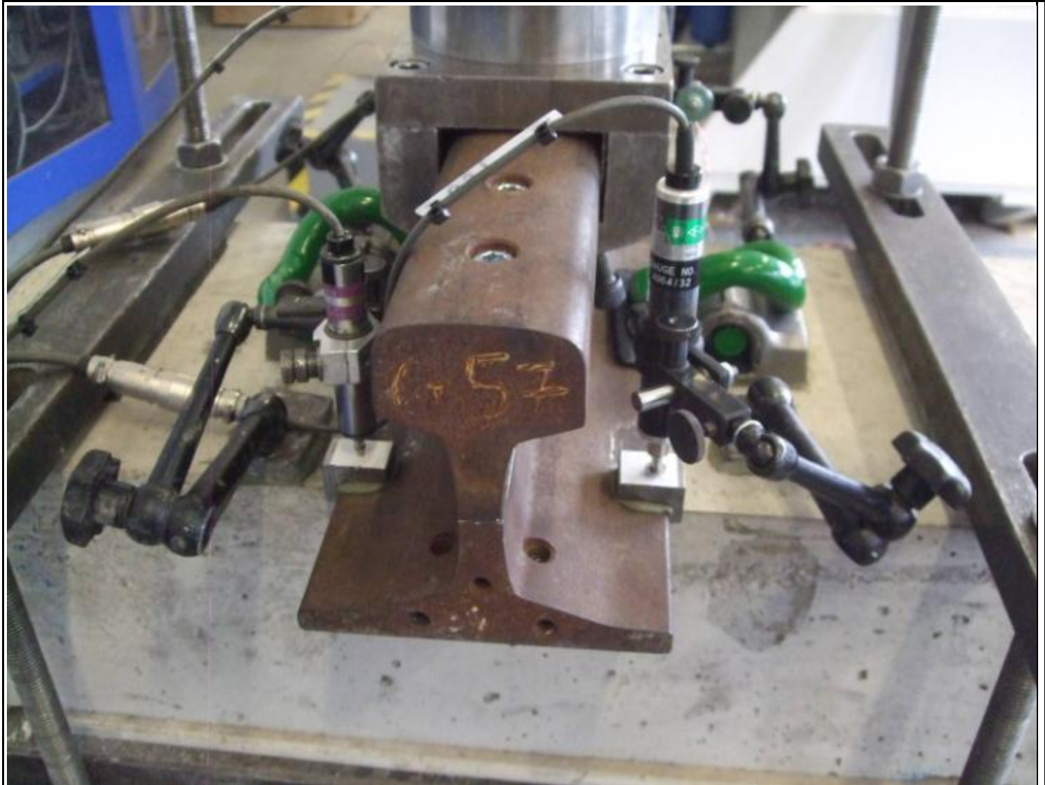
Clamping Force - Transducer Arrangement
