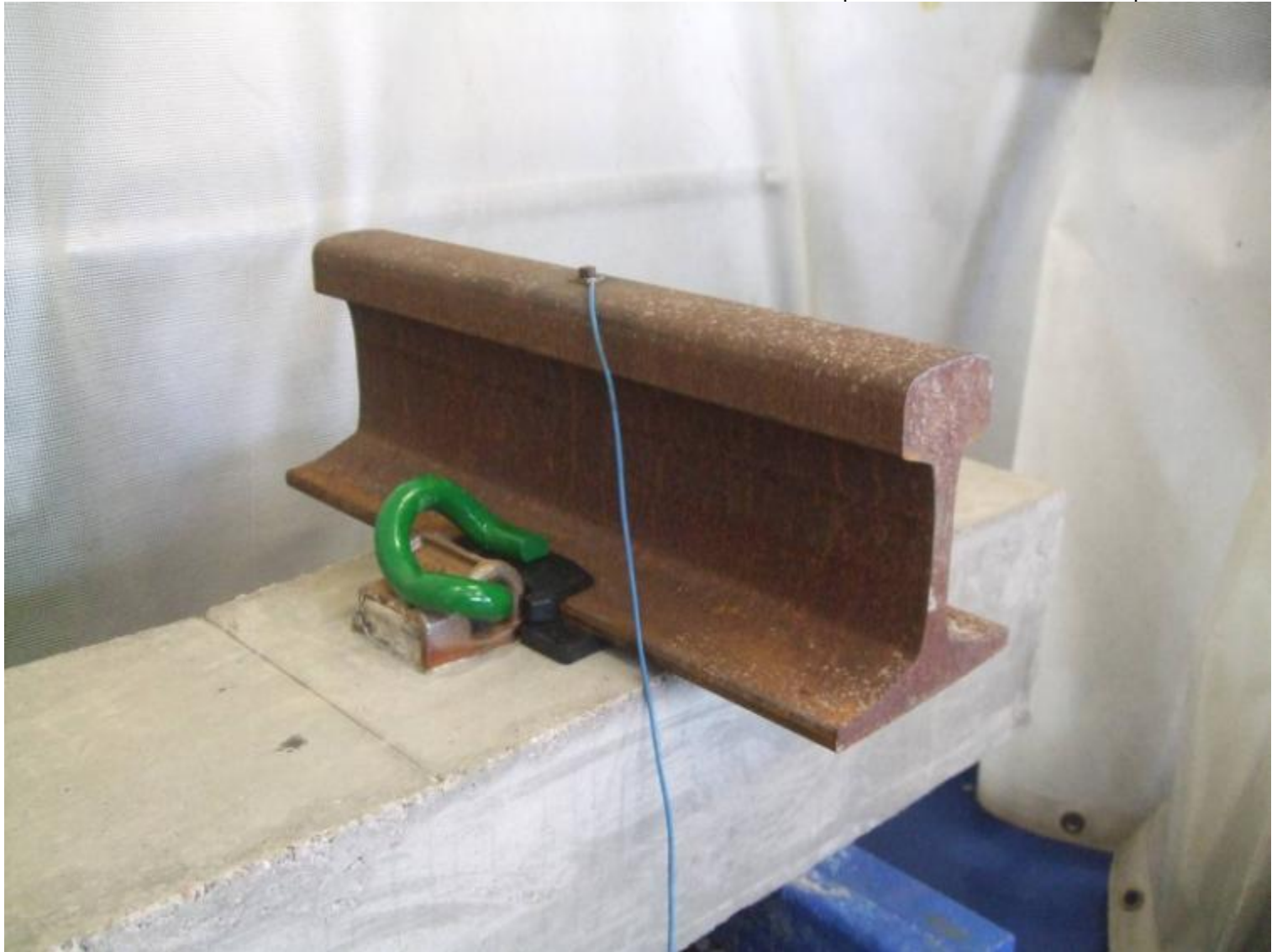
Electrical Resistance Test Sample
