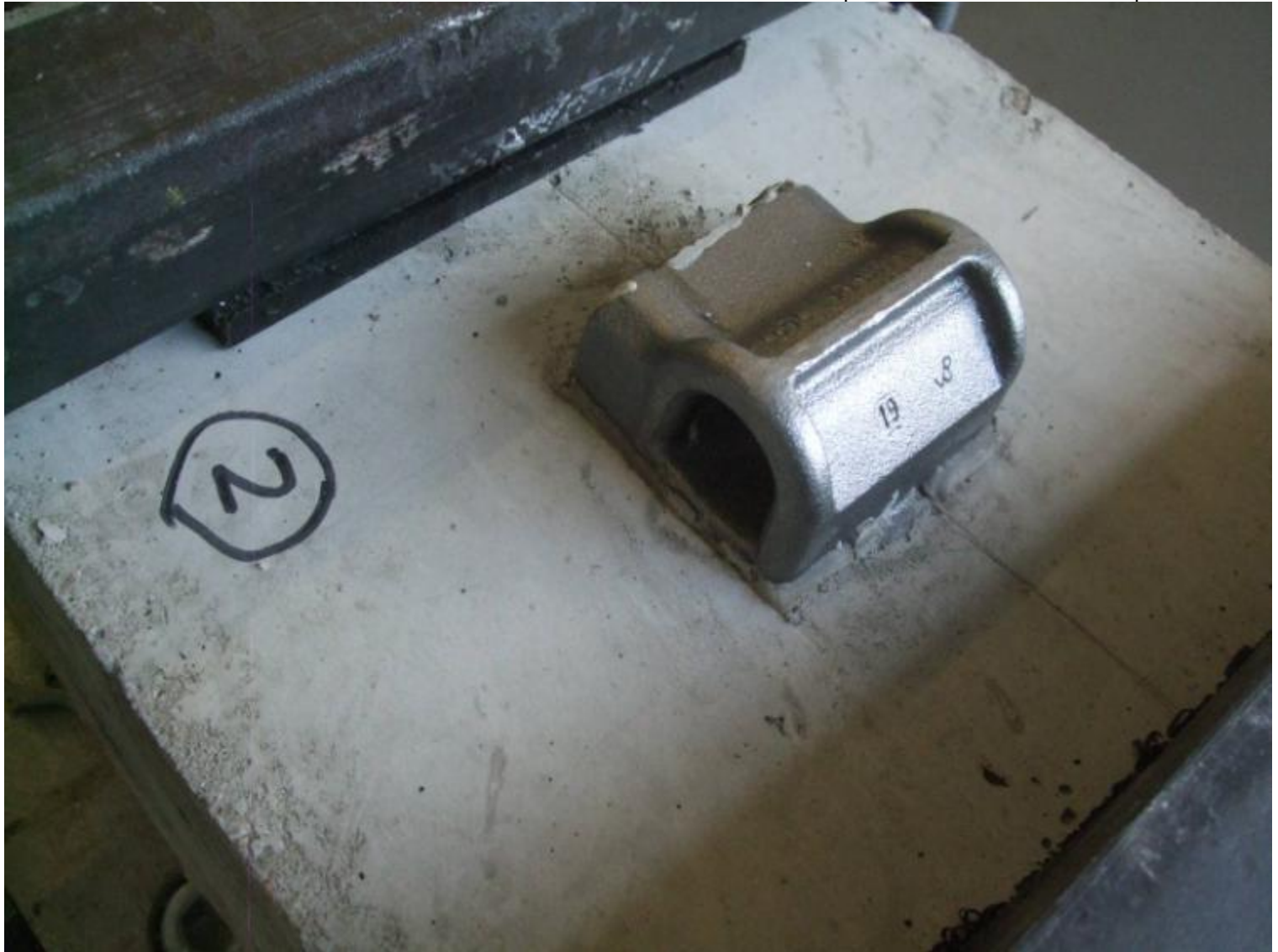
Vertical Load – Slab No. 2 Cast-in Component Surface Post test
