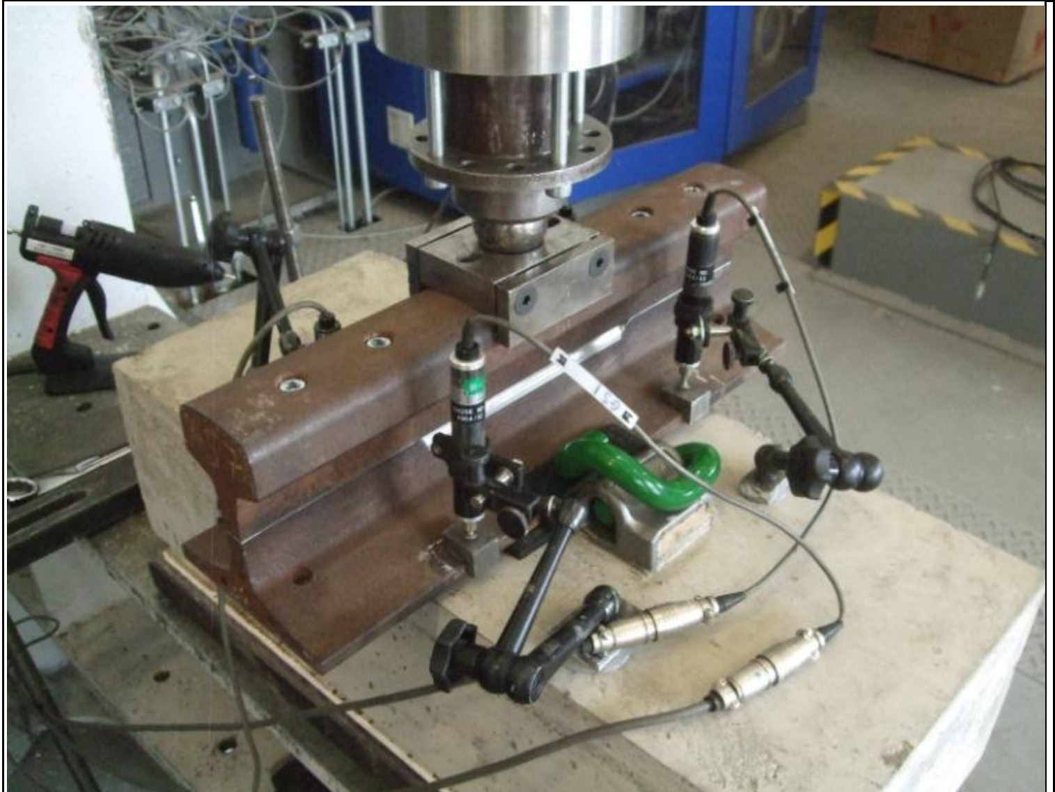
Vertical Stiffness - Transducer Arrangement
