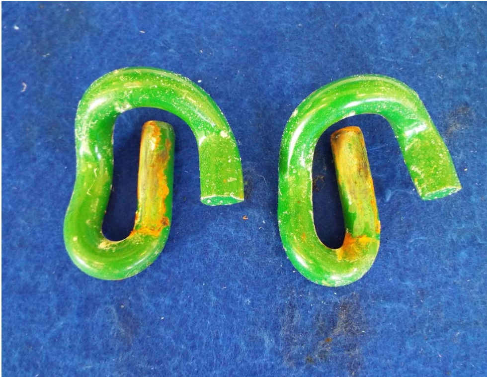
Figure A13: Rail clips upper surface following effects of severe environmental conditions test
