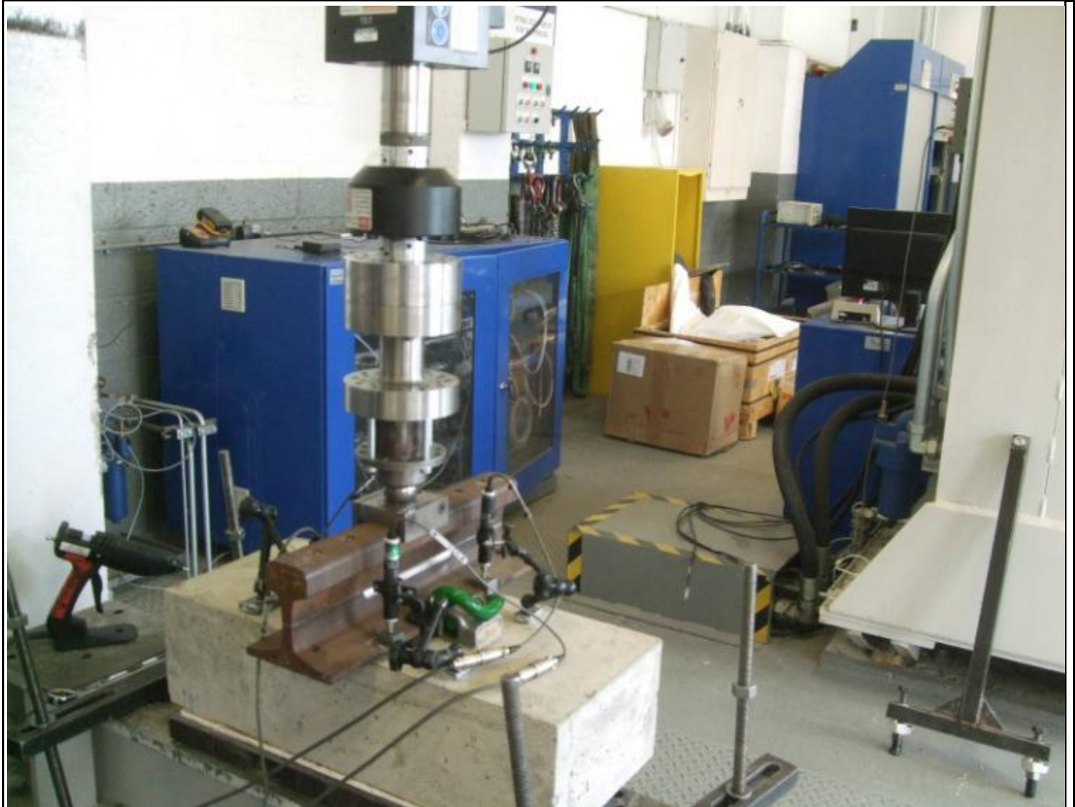
Vertical Stiffness - 100kN Actuator Test Rig & Transducer Arrangement
