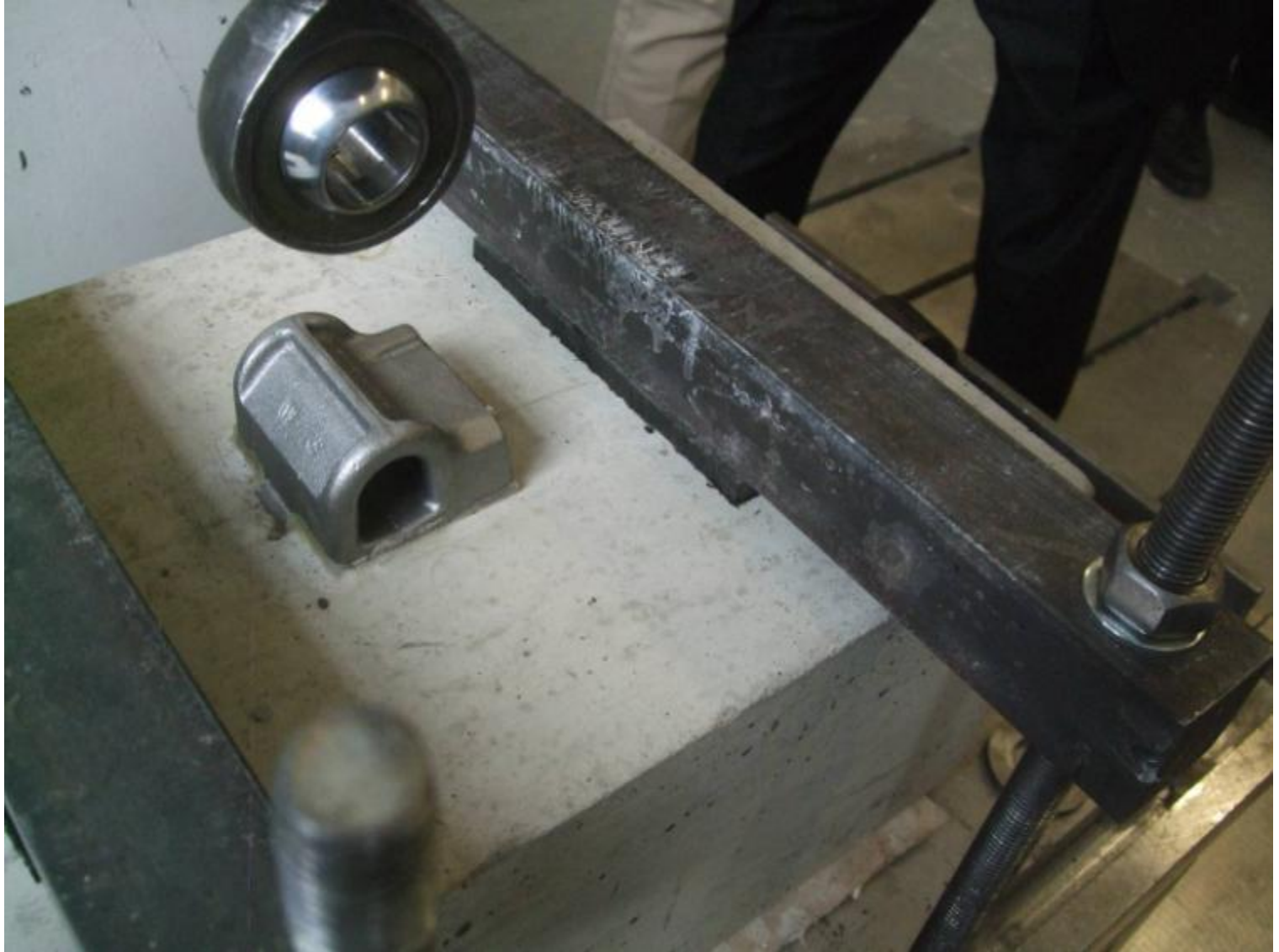
Vertical Load – Slab No. 1 Cast-in Component Surface Post test
