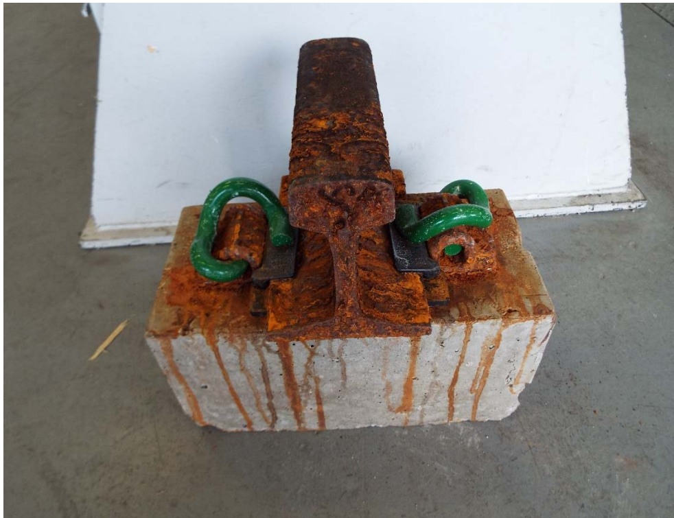
Figure A8: Assembly following effects of severe environmental conditions test
