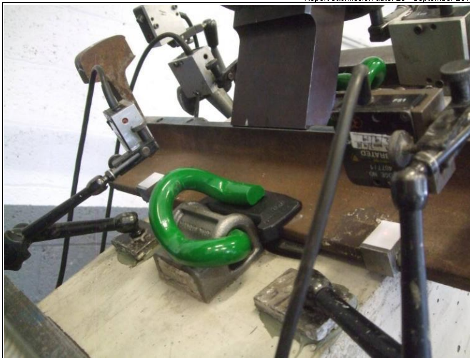
Repeated Loading Test – Laser Arrangement
