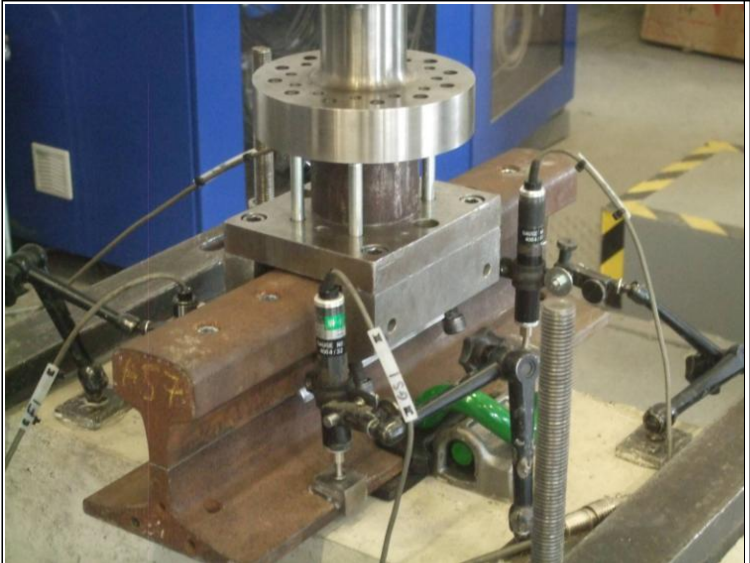
Clamping Force - Transducer Arrangement
