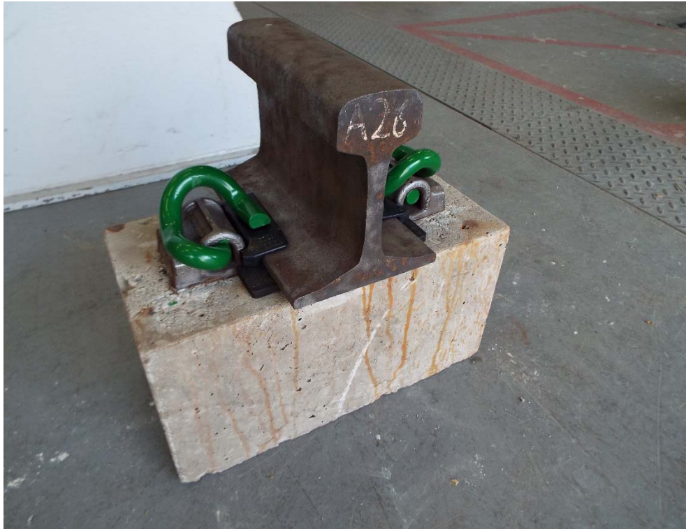
Figure A7: Assembly prior to effects of severe environmental conditions test
