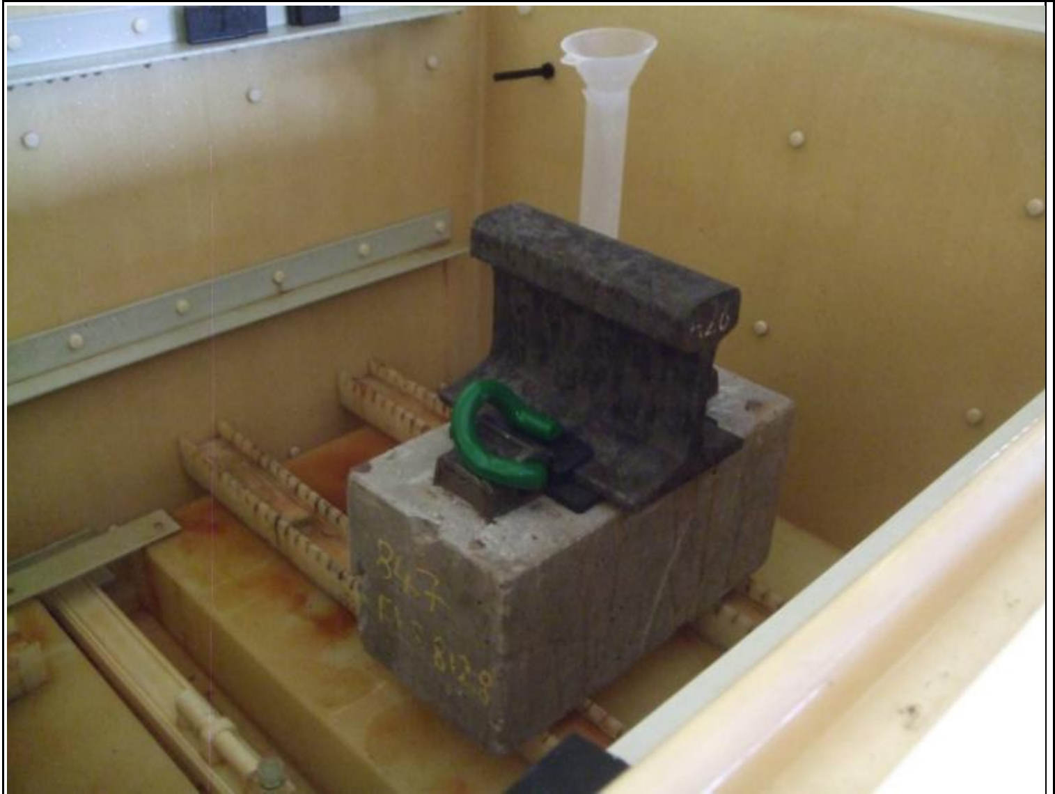
Severe Environmental Conditions - Salt Spray Cabinet
