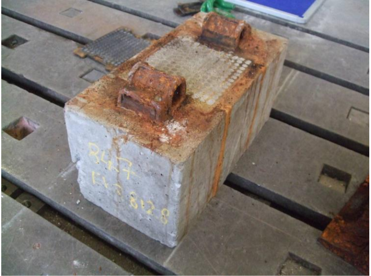
Severe Environmental Conditions - Slab after Dismantle
