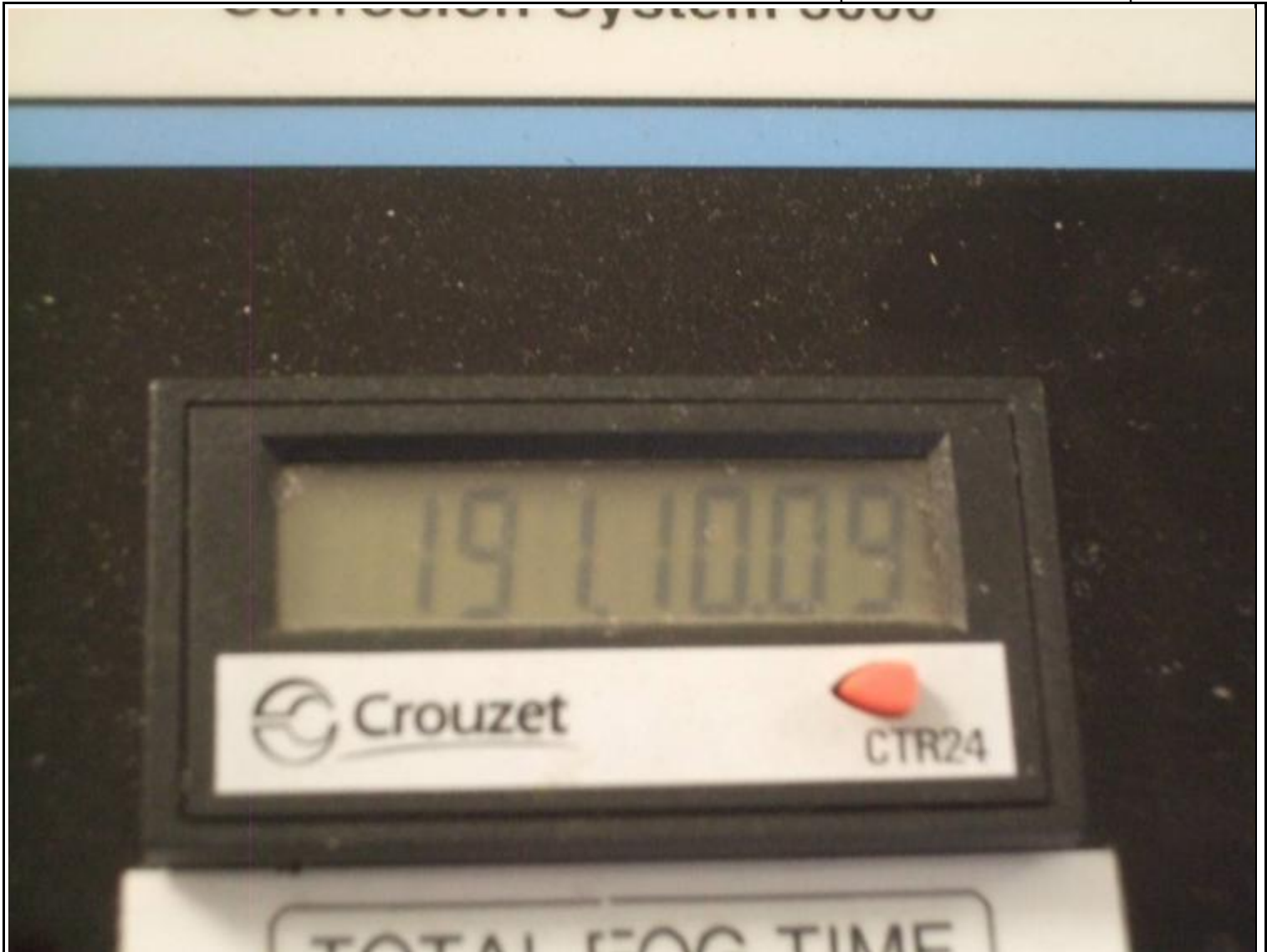
Severe Environmental Conditions Test started - Set for 300 hours [initial hour meter reading at start of test]
